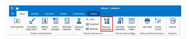
The most common use for an assembly is to group labor resources into crews (e.g., Pipe Crew, Concrete Crew); however, any resource (equipment, materials, etc.) may be grouped into an assembly. Utilizing assemblies allows you to estimate faster, since you can add and manage an entire group of resources at once.
